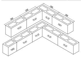
All units installed with a 10mm mortar joint in the perp ends. (Not included in block dimensions noted above)
