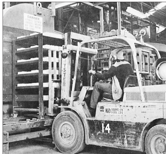
Figure 15 Forklift Truck Handling Racks of Blocks from Automatic Loading and Unloading Equipment, to and from Curing Chambers
