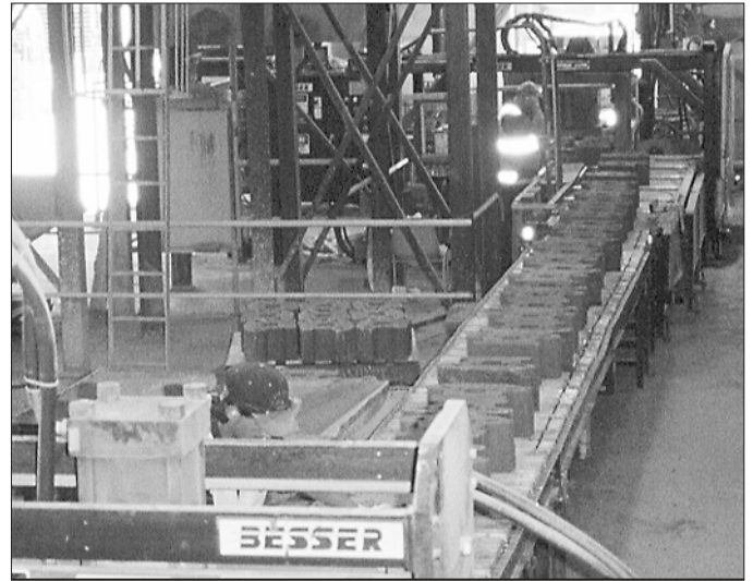
Figure 18 Cured Blocks on Machine Pallets being Transported to the 'Cubing' Machine after Unloading from the Kilns
