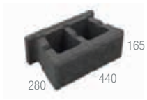
Modernstone® Standard Max Wall Height: 1050mm Units per m²: 13.77
